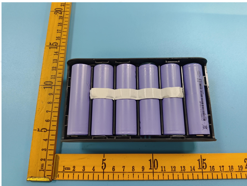
Fig.3 Internal view of Lithium-ion Battery Pack 锂离子电池组内部
