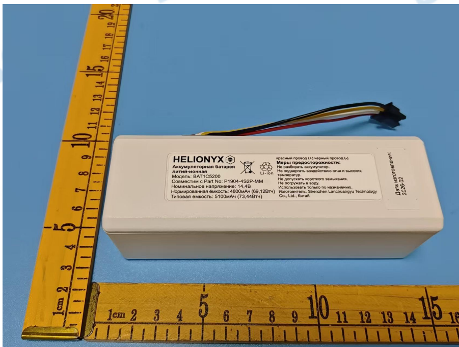
Fig.1 Front view of Lithium-ion Battery Pack 锂离子电池组正面
